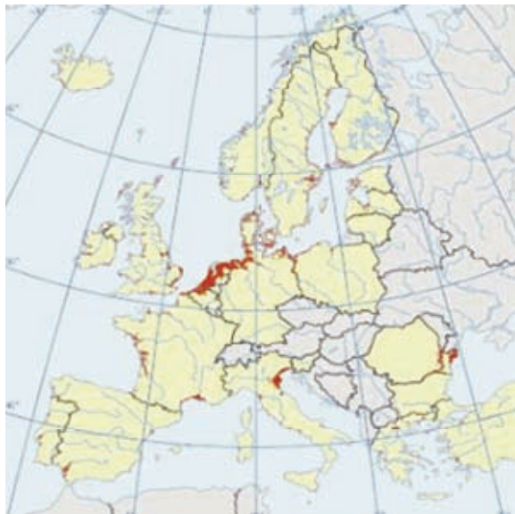
Figure 1.3.2. Low-lying areas along European coastline. Red surfaces are areas below 5m elevation. (source : EEA 2006)
